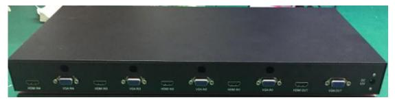
OUT: Main output. Achieve seamless switching or multi - screen display. DC 12V:Power interface.
